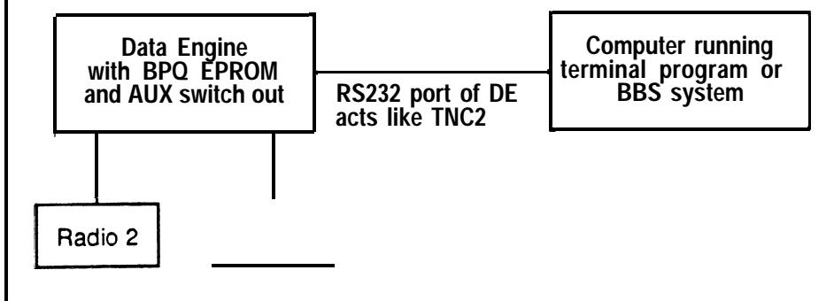
Frequently, we have the need for more than two radios in a single node, and this has been cumbersome in past implementations of node firmware. With the BPQ code running in the Data Engine, a simple press of the front panel AUX switch changes the serial port from a TNC-2 port to a KISS link, which may be connected to any KISS mode TNC. In this configuration (see figure 2), you can
