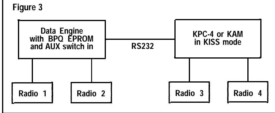
When using this method, all of the TNCs can be attached to a single serial port, such as the serial port of the Data Engine. A single diode is connected in the RXD line of each TNC, with the anode connected to the TNC and the cathode connected to the serial port of the com-
