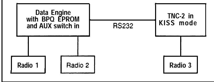
implemented dual port support using the Kantronics scheme. Since the KISS implementation as originally specified only uses the low nibble (4 bits) of the control byte to specify the function, the high nibble was used by Kantronics in version 2.84 and later of their firmware to address the two ports of the KAM and the KPC-4. If the high nibble was zero, then the unit would address one port, and if the high nibble of this byte was non-zero, it would address the other port.
