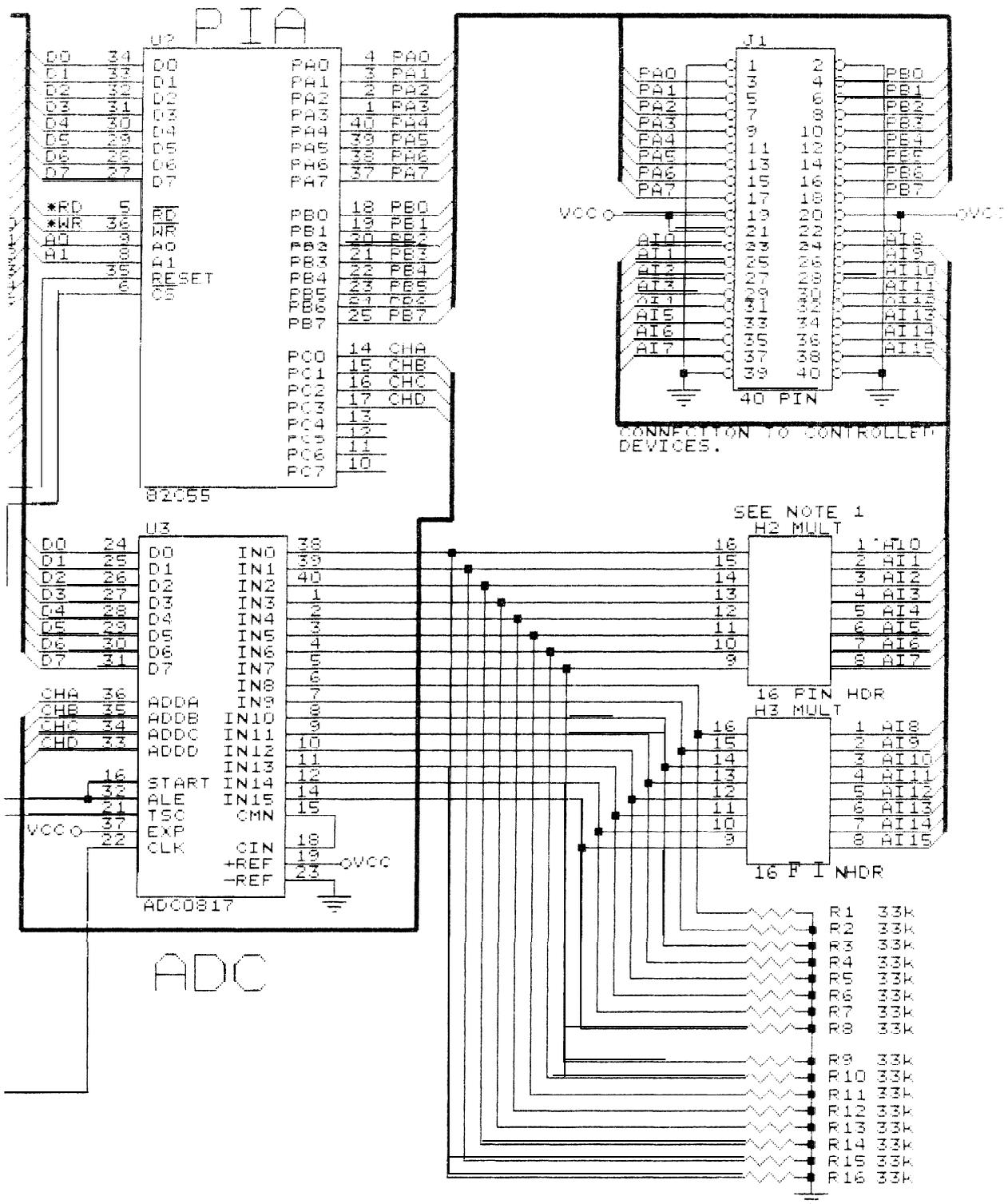
NOTE 1: MULTIPLIER RESISTORS WORK IN CONJUNCTION WITH R1-16 TO CHANGE THE BASIC 0-5VOLT RANGE I.E. A WIRE IN THE MULT POSITION IS 0-5VOLTS, AND A 33K RESISTOR IS 0-15VOLTS.
