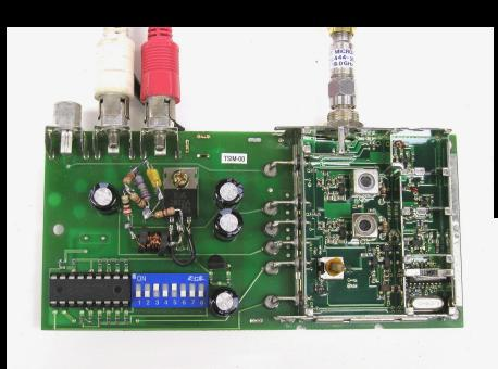
1200 MHz Transmit board with module cover removed
