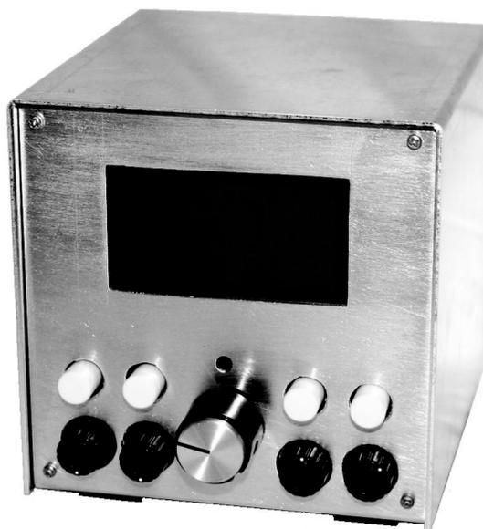
**Photo 1:** Cube prototype prior to application of black powder coating and white silkscreen labeling. Designed as initial companion to NUPSK digital modem, future growth will encompass modem functions and more.
