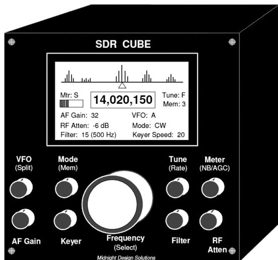
**Figure 1:** Graphic depiction of the completed SDR Cube Transceiver. Dimensioned at 4" x 4" x 4", design contains full user interface, DSP processing, I/O connectors on the rear panel, and 27 in<sup>3</sup> shielded space internally for Softrock.
