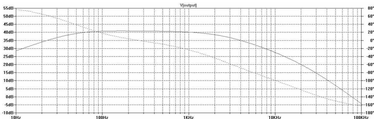
Figure 4: Op amp circuit frequency response.
