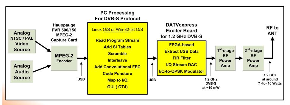
System Block Diagram for DATVexpress DATV Transmitter
