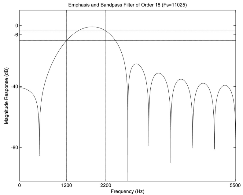
Figure 3 — This graph shows the response of a more practical low order (18) bandpass filter. It does not look nearly as good as the 180 order filter, and has a significant variation across the passband, it still emphasizes the high tone by about 6 dB.
