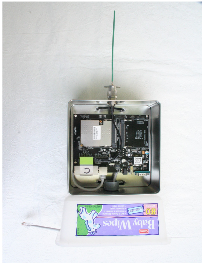
photo 3: router with quarter wave antenna and stand
