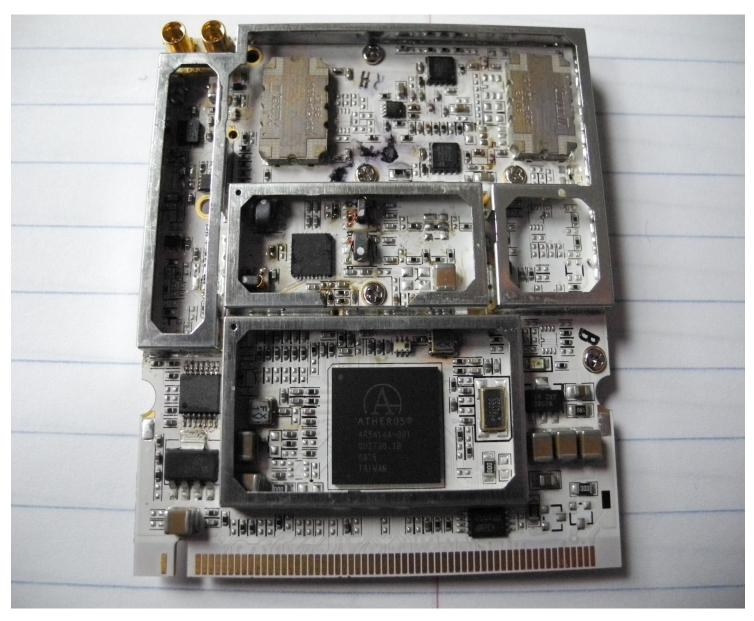
Doodle Labs DL435-30 with shield removed (KB9MWR photo)
