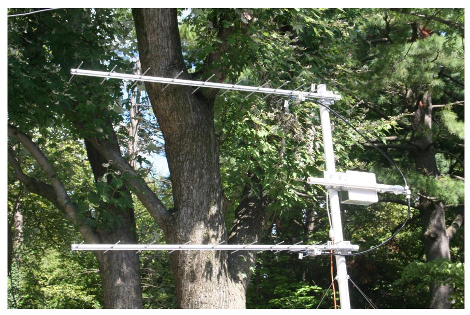
stack Yagi antenna array with router
