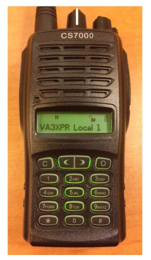
mockup of CS7000 narrow band data radio with GMSK, 4FSK modems
