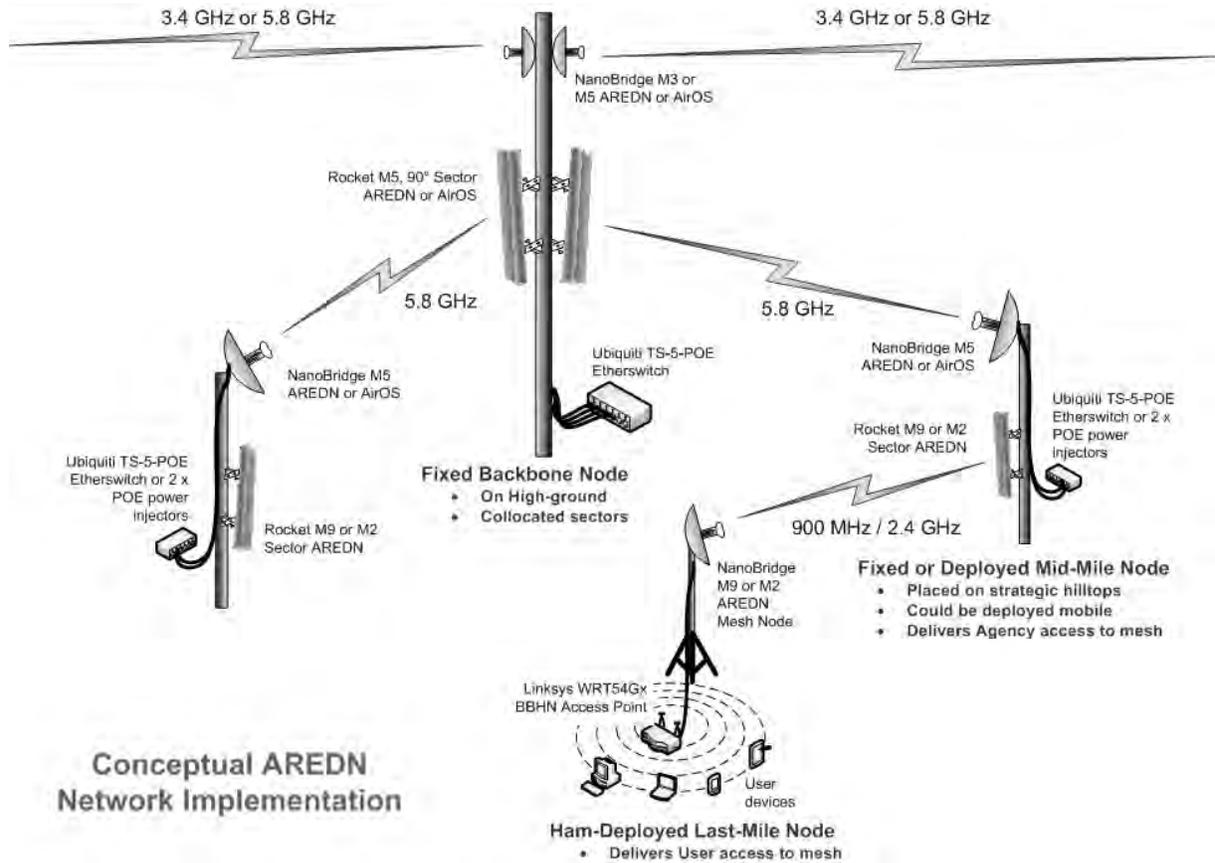
While the term “mesh networking” implies a peer relationship between nodes, a structured core of nodes is defined to establish an initial, predictable path for the network. Three node types are illustrated.
