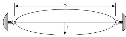
$$r \text{ (in feet)} = 36 \sqrt{\frac{D \text{ (in miles)}}{4f \text{ (in GHz)}}$$
