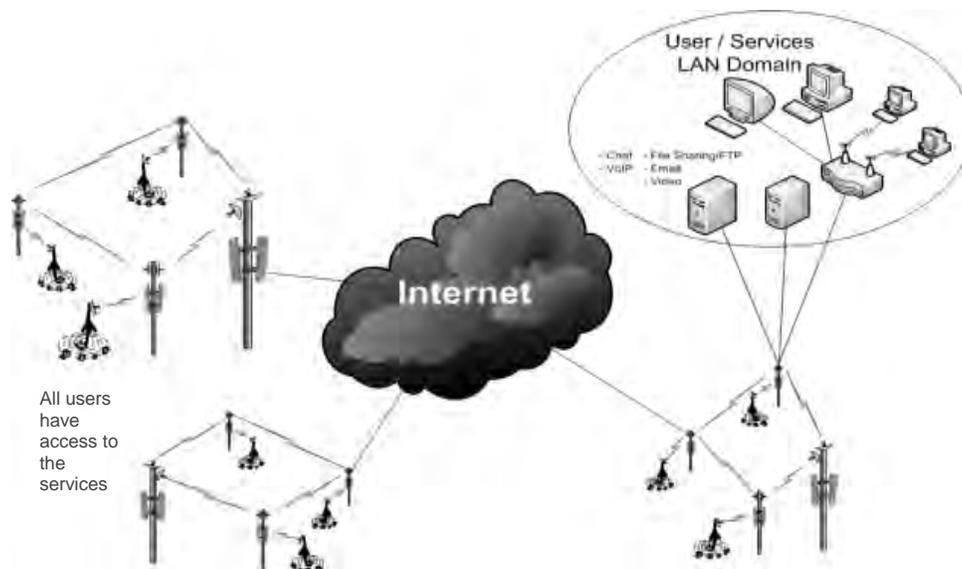
The interim solution AREDN has provided is based on Internet tunneling. This involves setting up an encrypted tunnel between one tunnel server-node and one node in each of the other mesh-islands. This has the effect of connecting all participating mesh-islands together in the same network. In doing so, you can gain the benefits of having completed the network and, at the same time justify the build-out of IP-based services for the users and demonstrate the utility to prospective customers.
