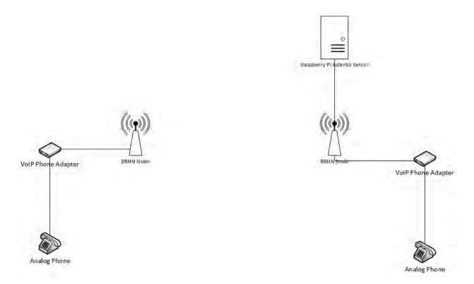
I was concerned that the VoIP phone adapters would not be able to easily communicate with the server due to DNS difficulties, but there were zero problems with DNS or DHCP in BBHN. Again, this reinforces that this system is designed for the common person.
