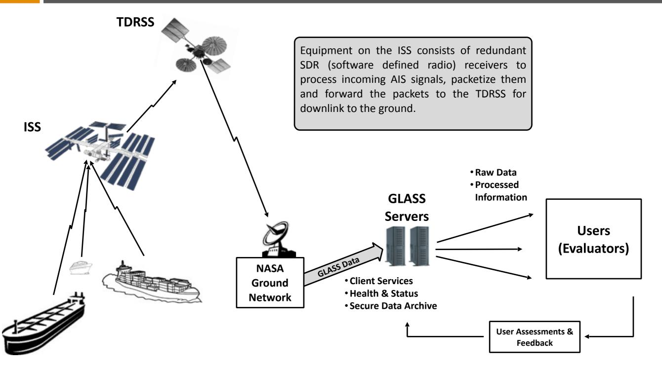
**ISS** – International Space Station **TDRSS** – Tracking and Data Relay Satellite System
