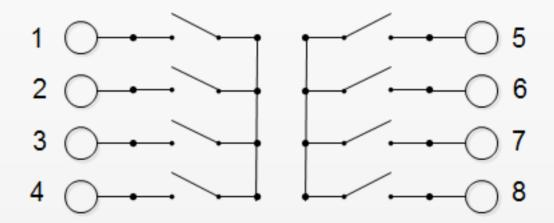
Two 4 pole "busses" Each switch controlled by logic signal
