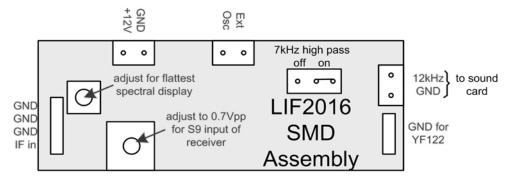
If the unit is placed in a transceiver with a YF-122 option filter, the pin header of the radio fits easily into the left and right PCB holes and slides down for a snug fit. For other receivers, the IF connection has to be made with a jumper. The +12V supply has to be picked off from a suitable spot inside the enclosure.
