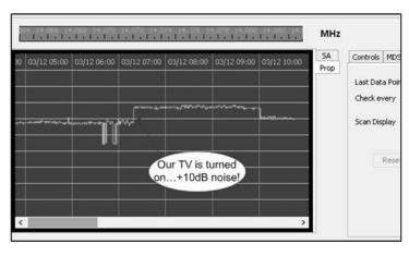
Measuring noise in the environment that surrounds the station is the first task of setting up an RF Propagation monitor. One of the biggest contributors of RF noise is the flat-screen TV. By monitoring the time noise occurs and vanishes one can pinpoint the location of offending units.
