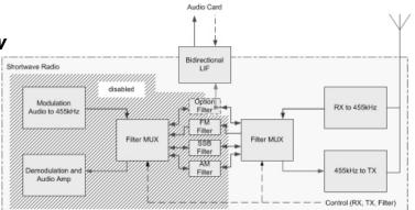
By processing the IF and not base audio, the MDSR software can perform a lot of the functions which most transceivers lack. As a second connection, the CAT cable is required to allow control of all functions of the host transceiver via the MDSR software. Thus, MDSR so completely controls the transceiver that it can be out of reach while operating.
