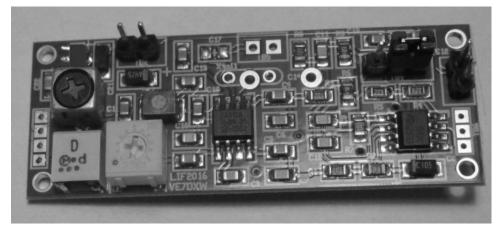
more amateur radio operators. It is mostly SMD and is assembled by robot. The design consists of two layers, and has over 95% ground plane coverage. Now the downconverter hardware is small enough to fit into most transceivers internally. It is actually pin-compatible with the YF-122 crystal filter that
