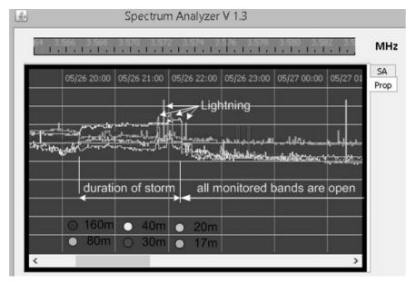
The buildup of energy in the troposphere was visible at least 2 hours before the storm hit (left of the "duration of the storm" marker). During the 2h storm the noise level of the 40m band jumped way up. In this particular storm the lightning passed last, mostly seen in the green spikes (80m). Just after 22:00 a big lightning strike makes even the 17m band jump. At 22:15 the noise of the 40m band drops almost immediately even though the storm was only a few miles away. And then something
