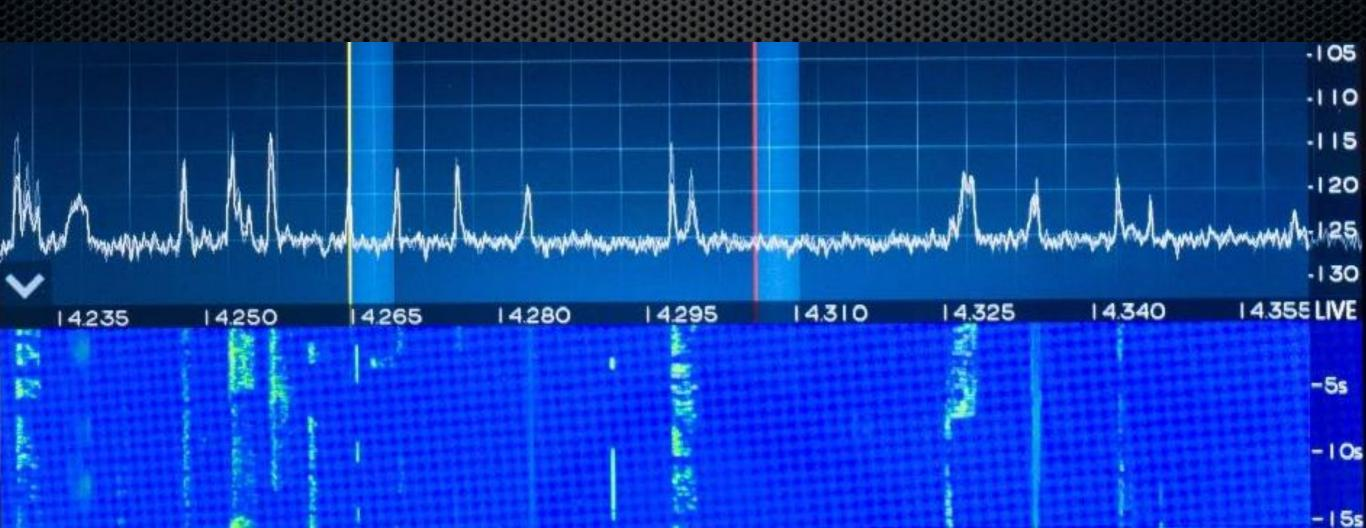
I looked up the ADC in my direct sampling receiver, it says 16-bits with an ENOB of 12.3 bits and 74dB SNR. I know there are 6dB per bit of dynamic range. 12.3 x 6 = 74. Heck, even if I could use all 16-bits, 16 x 6 = 96dB. My radio manufacturer says it has 105dB of 3rd order dynamic range.
