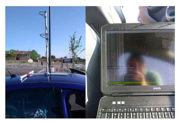
Figure 10: Testing TX/RX Communication in Belen, NM. The vehicle was not moving for these tests, and the mobile double-stacked halo antenna was used.
