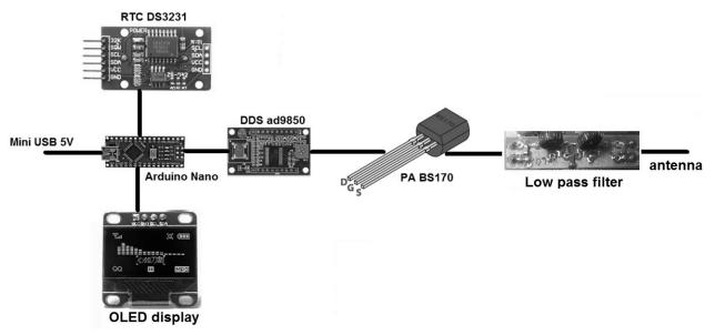
The real-time clock synchronizes Arduino to transmit every even minute. The Oled screen is optional and simply displays the time. DDS (Direct Digital Synthesis) generates an RF signal. The transistor BS170 is used as a class E amplifier and requires a low-pass filter.
