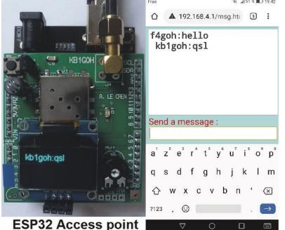
We notice that the processor has 2 cores. Core 0 handles digital processing and thus RTTY decoding while core 1 handles the main loop and the web server.
