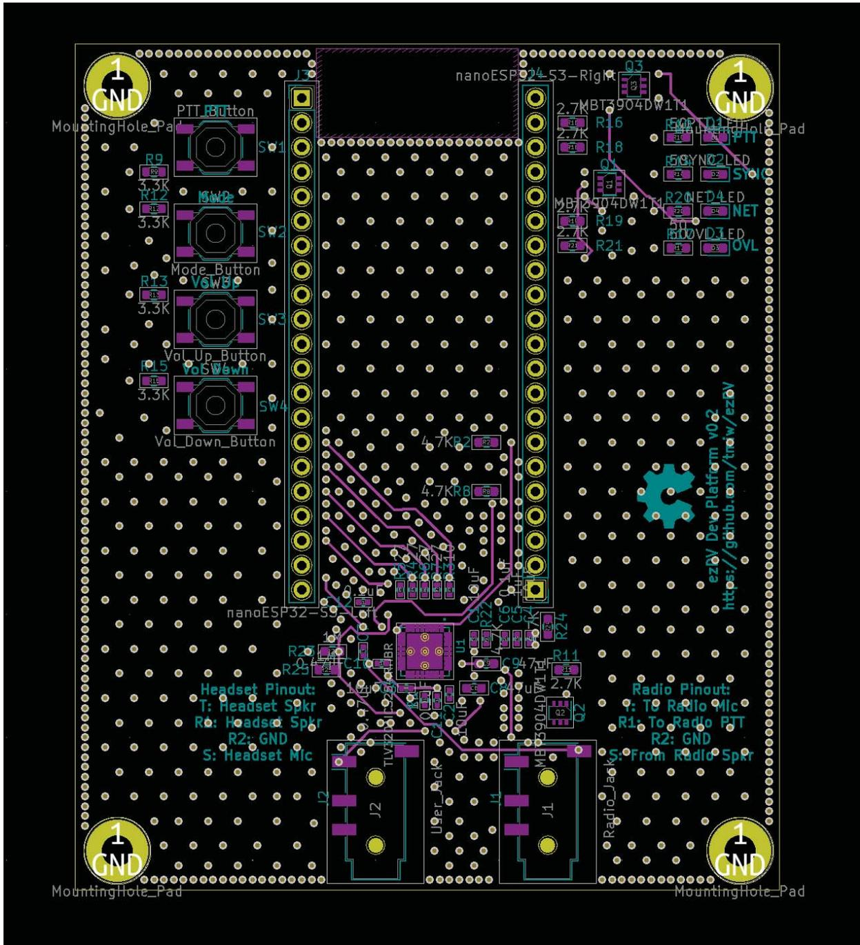
Figure 5: The bottom signal layer of the ezDV PCB.
