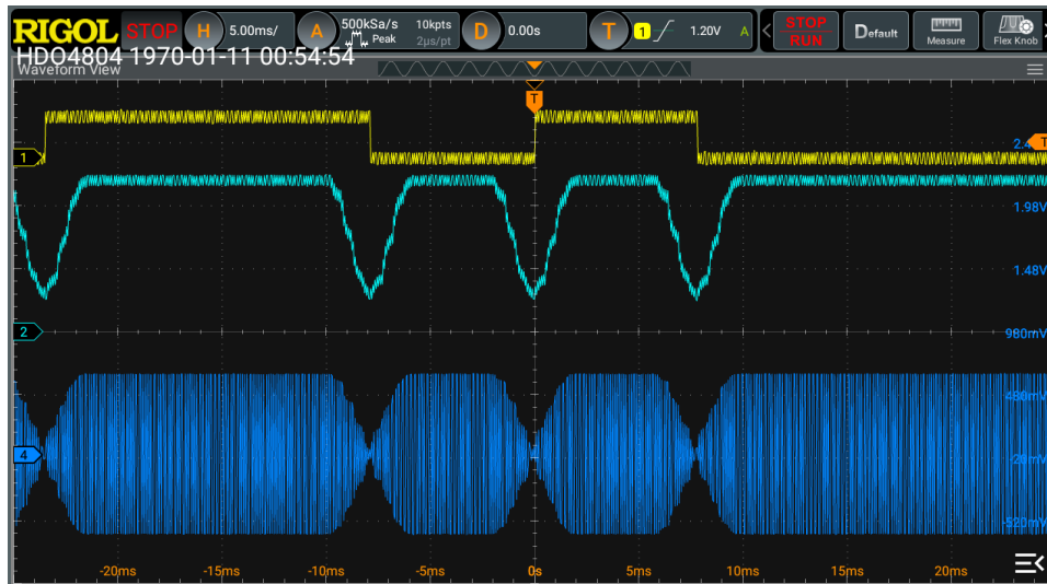
The modulated BPSK carrier envelope during phase transition
