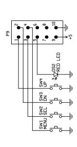
HOTE: A 14 CONDUCTOR CABLE WITH A 14X1 CONNECTOR ON BOTH ENDS IS SUPPLIED WITH THE KIT. THIS PLUGS TO J10 ON THE ON THE MAIN BOARD.
