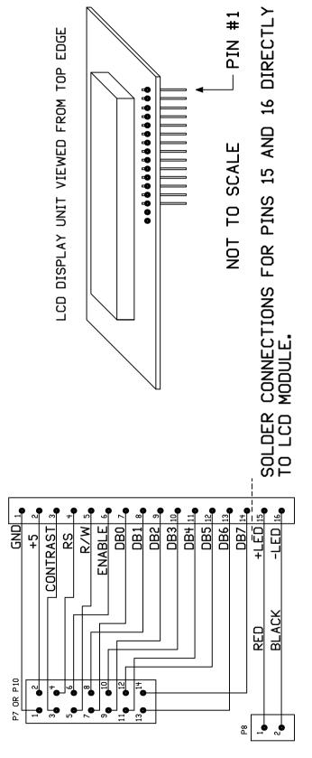
WIRING HARNESS FOR LCD MODULE
