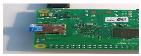
Figure 3: SD Card Installed in Pi
