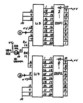
$D_1, D_2 = 1N4148$   $U_1, U_2 = LM1458$   $U_3, U_4 = LM3914$ DSP1. DSP2 = MV5310C +V = + 12V
