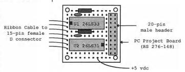
RS-422 Interface Daughter Board for TAPR 9600 bps Modem (drawing is not to scale)
