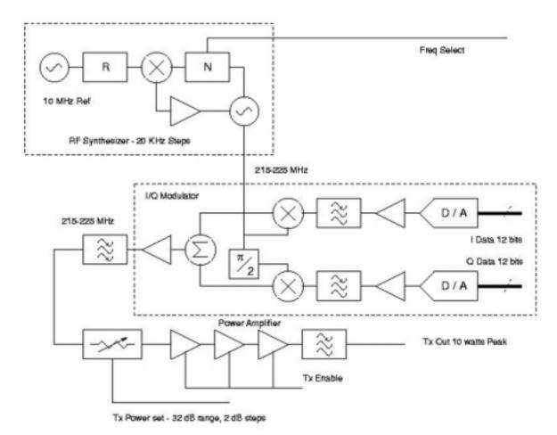
Transmitter Functional Block Diagram
