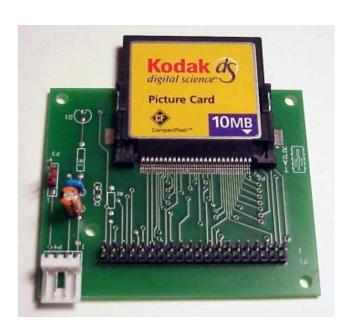
Figure 2: The TAPR CompactFlash Adapter Card, with a 10-Mbyte Kodak CompactFlash card. The adapter card turns the CompactFlash card into a 100% IDE compatible solid-state hard disk, able to operate from -25(C to +75(C, perfect for those cold mountaintops and hot deserts.
