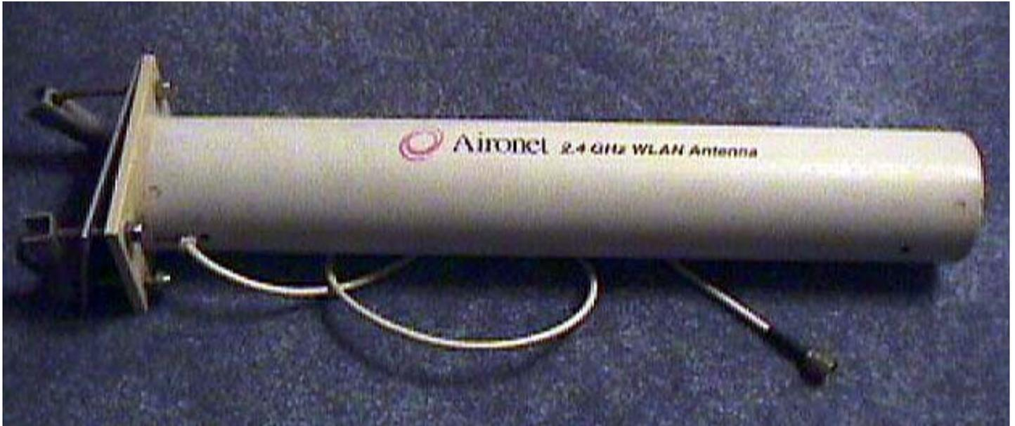
FIGURE 1: THE AIRONET 2.4-GHZ WLAN ANTENNA INSIDE ITS HOUSING.
