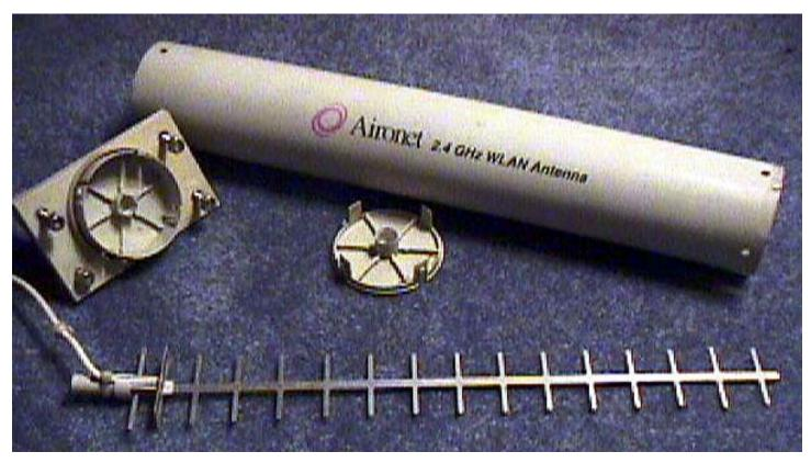
FIGURE 2: THE ANTENNA REMOVED FROM THE HOUSING. IT IS STAMPED FROM A SINGLE PIECE OF 1/16-INCH ALUMINUM SHEET.
