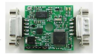
**Software DCD –** With this option enabled the T2 can be operated with the radio's squelch open, allowing faster acquisition of incoming packets. A mute output will also be available for Mic-E repeater operation.
