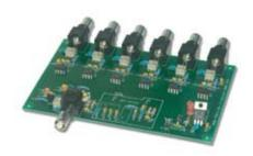
onboard LM7805 regulator and operates from 7-15 VDC. Current drain at 13.8 volts ranges from 70 to 250ma depending on load and duty cycle.
