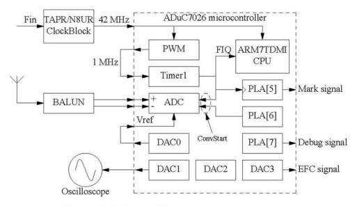
Figure 8. Blockdiagram of the receiver hardware.
