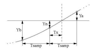
Figure 32. Interpolating the zero crossing
