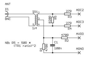
Figure 7. Antenna Balun Schematic
