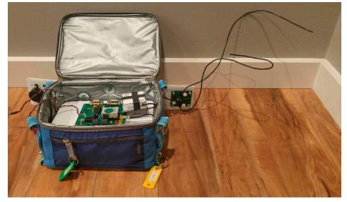
One of the APRS Trackers used to record eclipse data. Notice that an antenna boom (made from Corroplast) is bolted to the back of the lunch bag. You'll also see that four nylon straps are bolted to the corners of the lunch bag. This is where tether lines attach the tracker to the parachute's shroud lines.
