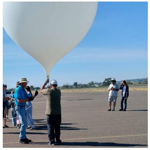
About one dozen people helped raised this balloon. It's around seven feet tall and filled with enough hydrogen to lift 15 pounds (twelve pounds for its payload and three for the proper ascent rate).
