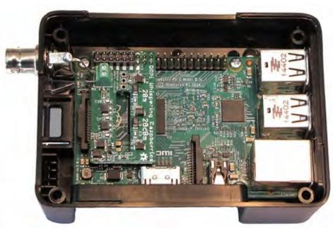
Figure 1. Raspberry PI 2 with QRPi Shield installed on left.
