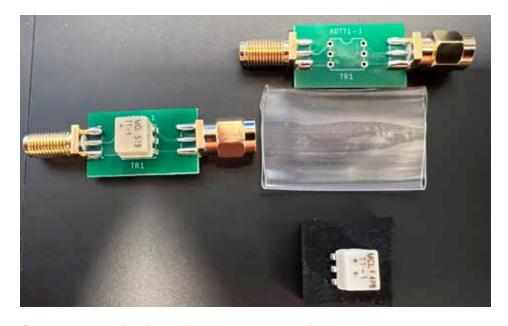
from eBay and other Chinese sources. The ones we've seen use a different, less expensive, type of transformer that is not as effective at blocking common mode noise. The T1-1's design ensures minimum capacitance between the windings, maximizing common mode rejection.
