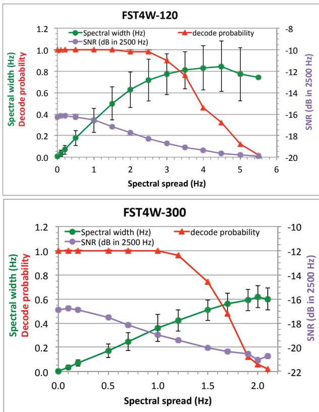
Figure 5. Variation of spectral width, decode probability and SNR with spectral spread from 50 runs of the *fst4sim* model at each value of Doppler spread for -120 upper, and -300 lower. The bars on spectral width are at +/-2.5 times the standard deviation, that is, 99% of the values lie within the interval.
