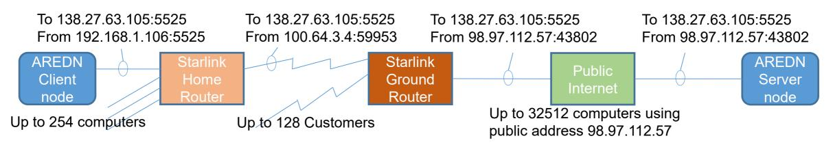
The Client→Server works because the To: address and port number are unaltered from AREDN client towards the AREDN server. The Internet knows how to route the packet to the AREDN server (To address).
