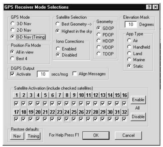
Figure 5. TAC32 GPS Mode Receiver Selections
