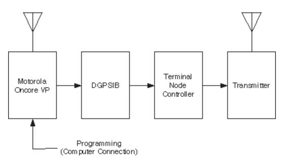
Figure 4. Basic Reference Station Block Diagram
