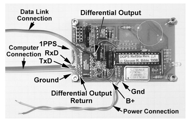
Figure 1. Location of Power and Data Connections
