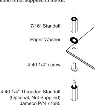
Figure 3. Mounting Hardware
