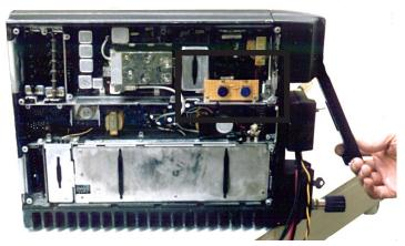
Picture of Perf Board for TAPR/G3RUH Modem modification. Mounted in Upper Right Corner.
