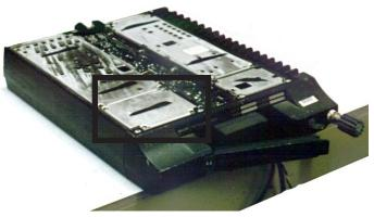
Refer to the audio squelch board layout for the location of JU201. If JU201 is not installed, add this jumper using a short length of insulated wire. This finishes work with the audio squelch board. When you place this board back in the radio, be sure that the 6 pins that plug into the audio power amplifier board (2 transistors on a heatsink mounted to the side of the radio) mate correctly.
