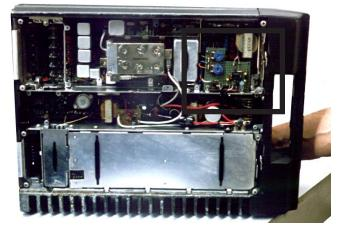
Picture of Perf Board for TPRS Modem modification. Mounted in Upper Right Corner.
