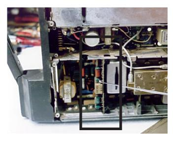
2. Remove the TX PL encoder (if installed). This board plugs into the excter board from the bottom side of the radio. The encoder board location is also shown in the bottom view of the radio.
