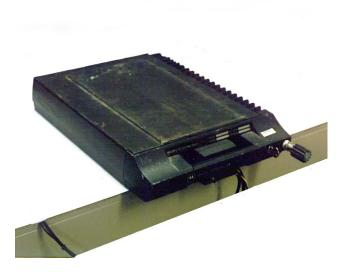
The transmitter employs a hetrodyne exciter. Receiver oscillator injection is mixed with the signal from an offset oscillator to generate the transmit frequency. The offset oscillator is varactor modulated for true FM.
